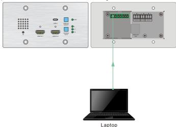
When control the far-end third party device from local control device (e.g. PC), connect the PC to the RS232 port of the switcher, and then connect the third party device (e.g. projector) to the RS232 port of receiver. The connection diagram shown as below:
