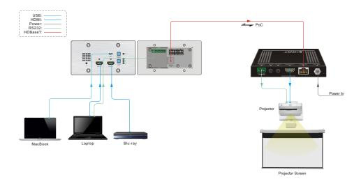
**Note:** We recommend CATx cabling with alien crosstalk prevention technology to ensure the performance of HDBaseT link.
