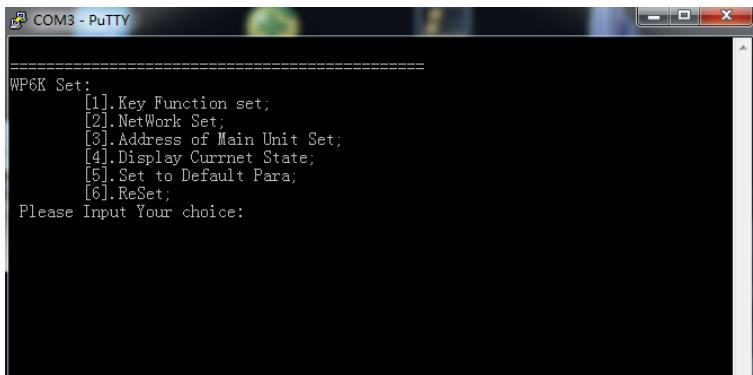
There are 6 menu can be chosen: [1] Key Function Set; [2] Network Set; [3] Address of Main Unit Set; [4] Display Current State; [5] Set to Default Para; [6] Reset.
