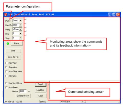
Set the parameters (baud rate, data bit, stop bit and parity bit) correctly to ensure reliable RS232 control
