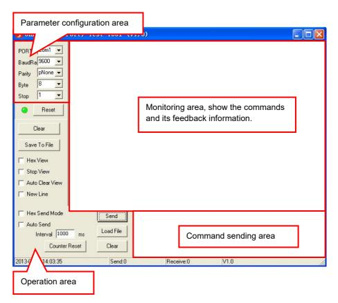
Please set the parameters of COM number, baud rate, data bit, stop bit and the parity bit correctly, and then you will be able to send command in command sending area.
