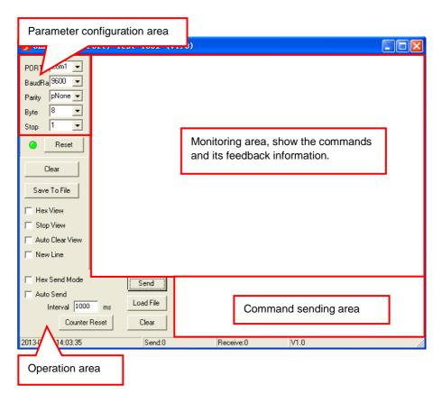
Please set the parameters of COM number, bound rate, data bit, stop bit and the parity bit correctly, and then you are able to send command in command sending area.
