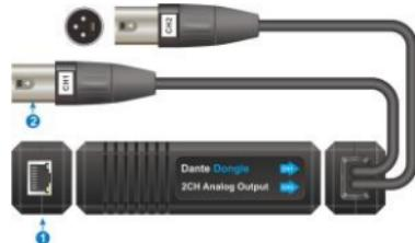
① **RJ45:** Dante network communication port. Green steady light indicates system ready; yellow flashing light indicates link/data traffic. The green light will flash to identify the device when clicking the Dante Controller "Identify" button (an eye-shaped symbol) on the host computer.
