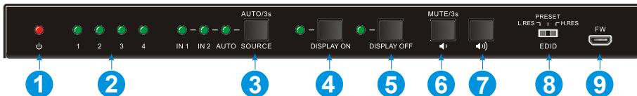
① **POWER LED:** The LED illuminates red when power is applied.
